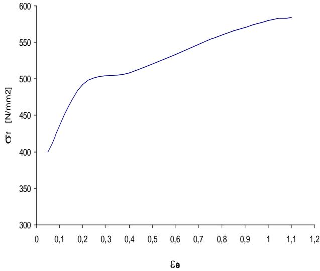
Fig. 1. Change of flow stress ( $\sigma_f$ ) as a function of effective strain  $\epsilon_e$
