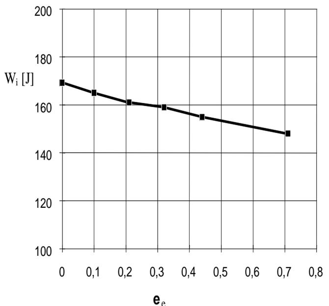
Fig. 3. Impact toughness ( $W_i$ ) as a function of the effective strain ( $\epsilon_e$ )
