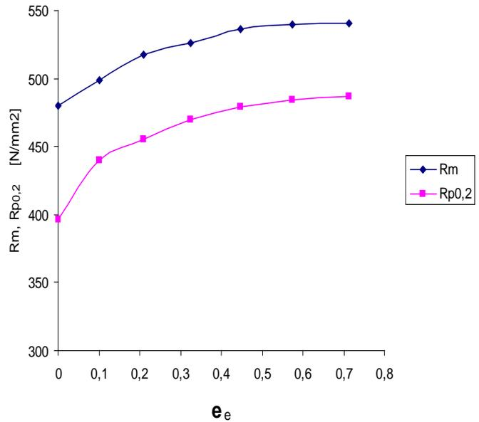
Fig. 2. Tensile strength ( $R_m$ ) and yield strength ( $R_{p0,2}$ ) as a function of the effective strain  $\epsilon_e$
