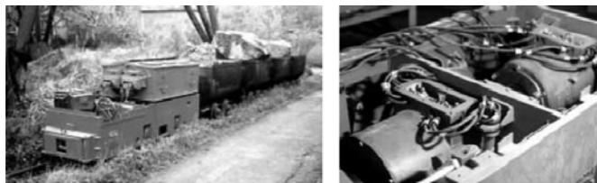
**Fig. 2** Common view of the traction locomotive and placement of the electric motors.
