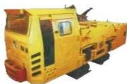
**Fig. 1** Contact mine electric locomotive of type 10KR.
