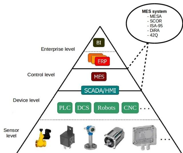
Fig. 3 MES in standard automation model.
