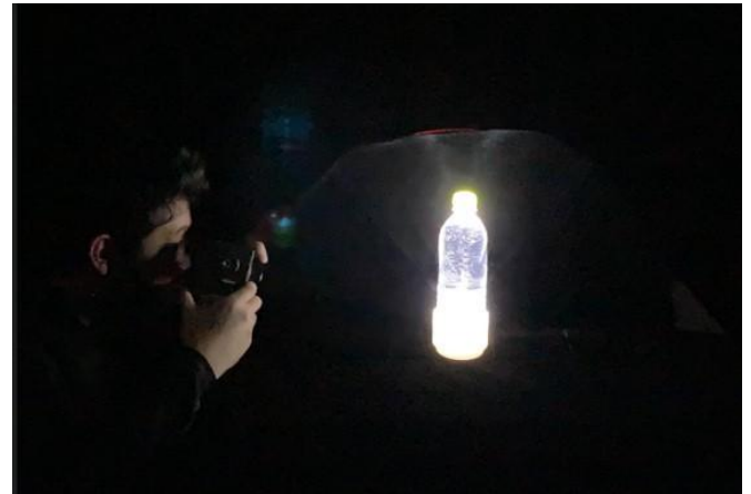
Fig. 9 Measurement. Using a guide attached to a protractor, the measurer positions the lens of the luminance meter so that it is equidistant from the LED and measures the luminance
