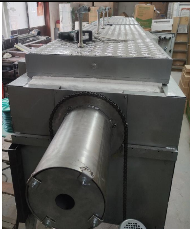
Fig. 3. Modified prototype of a facility for obtaining foam granules of composite material.
