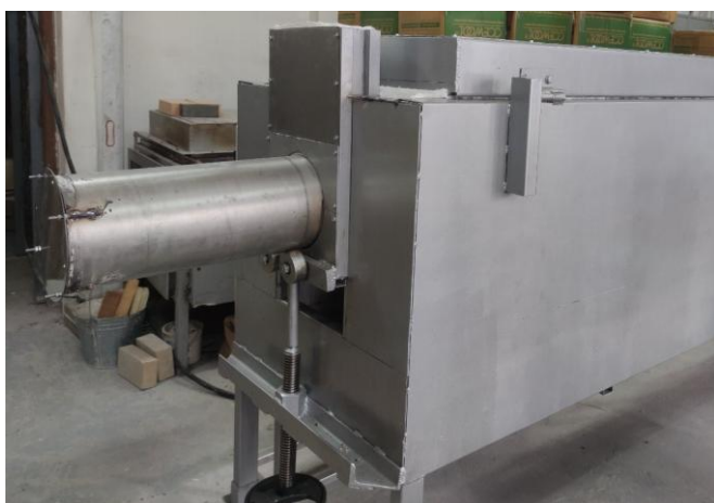
Fig. 2. Modified prototype of a facility for obtaining foam granules of composite material.
