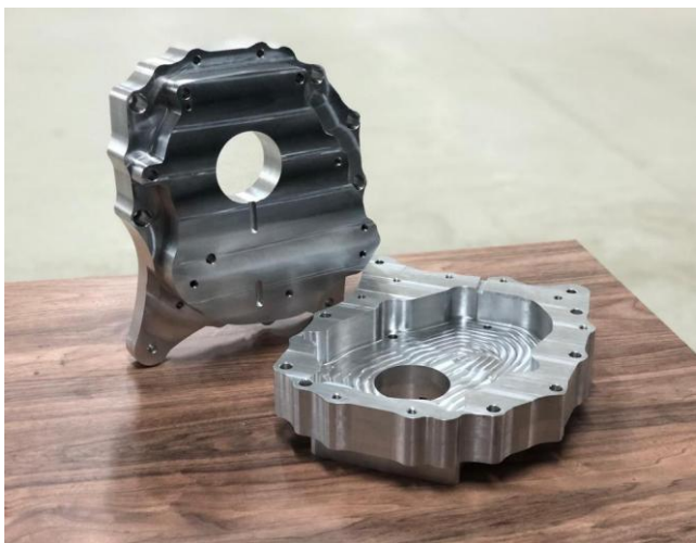
Fig. 7 CNC machining of the counterpart (up), Final counterpart produced by AL 7075-T6 (down)
