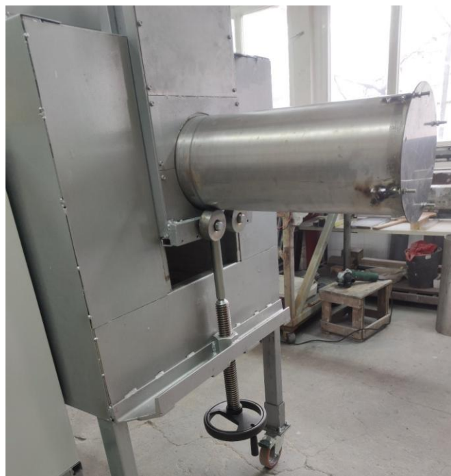
Fig. 4. Modified prototype of a facility for obtaining foam granules of composite material.
