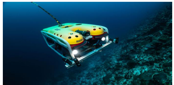
Figure 1. Saab Seaeye Falcon fitted with a special stereoscopic camera array. Nekton Maldives Mission © Nekton 2022.
